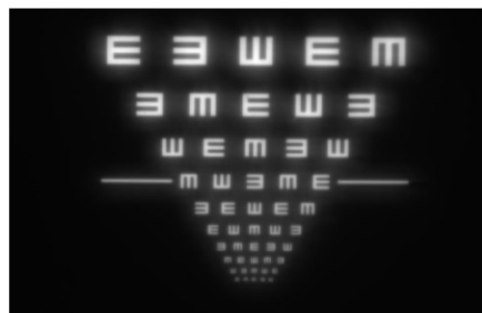
MODEL EYE (+0.18 \mu M SPHERICAL ABERRATION) †
